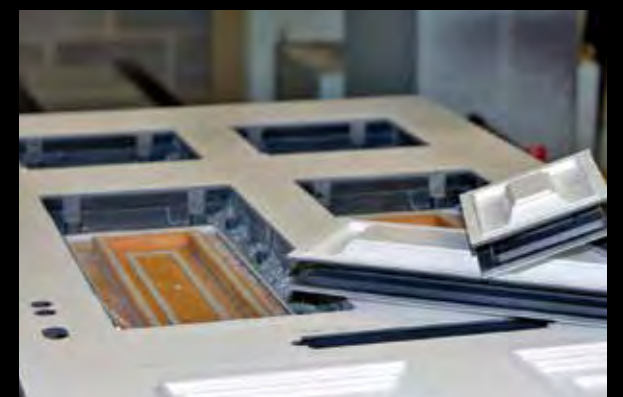
Door after routing operation
